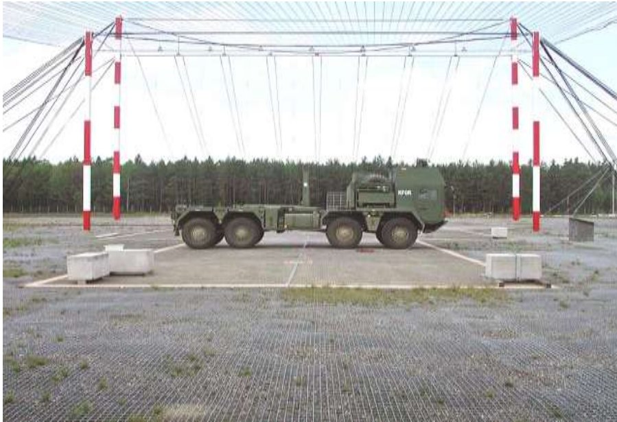
NEMP-Generator with Strip-Line
