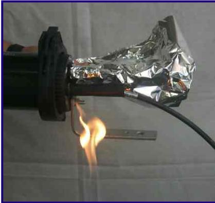
**19** Shrink down the heatshrinkable sleeve onto cable. Use aluminium foil to protect other cables and entry ports. Allow the heatshrinkable sleeve to cool completely.
