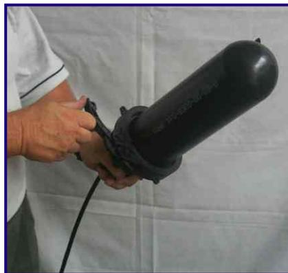
**23** Fit and tighten the swing clamp.
