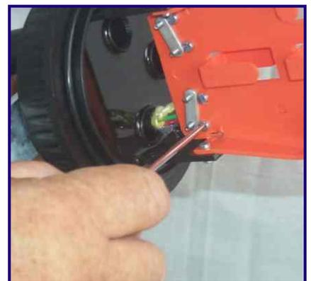
**15** Position the open end of the cable A level with the entry port and tighten GRP link screws.
