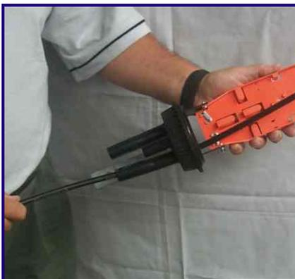
**4** Pass cable through open cable entry port, leaving sufficient length of cable for splicing  $\pm 1.5M$ .
