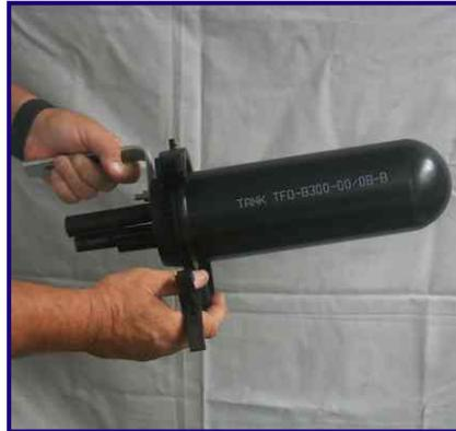
**2** Open swing clamp and remove closure body.
