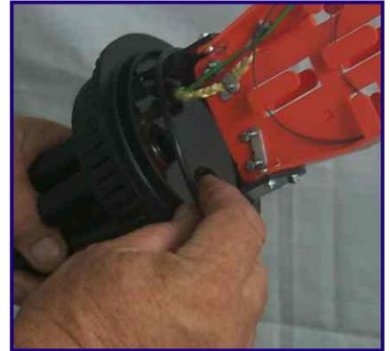
**21** Check that the O-ring is correctly seated and that the sealing surfaces on the base and body are clean and damage-free.
