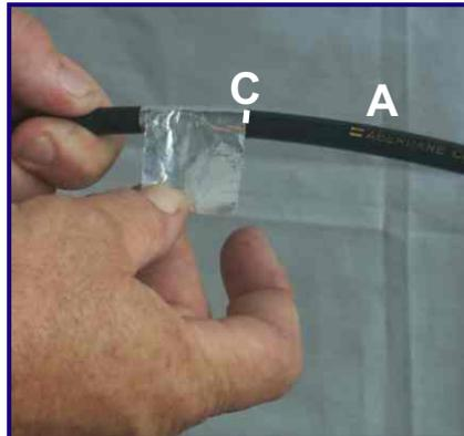
**11** Wrap aluminium tape around cable at C towards B.
