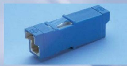
The E-2000<sup>™</sup> compact adapter is space saving and comes equipped with a **quick-lock mechanism**. This compact version of the standard E-2000<sup>™</sup> connector does not require screws or other fastening devices. The fixing spring shackles are integrated in the adapter housing and are suited for front plates with a wall thickness of up to 1.6 mm and SC standard cutouts.
