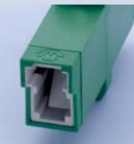
The integrated full-metal diaphragm in the adapter protects from emerging laser light. The full-metal safety cap in the connector opens and closes automatically. The safety cap has an integrated spring safety device which prevents the ferrule end faces from becoming dirty or damaged.
