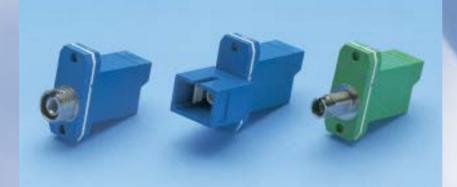
E-2000<sup>™</sup> Hybrid Adapters allow connections between the E-2000<sup>™</sup> connector and FCPC, FLSA or FSC connectors. All Hybrid Adapters are equipped with a slotted zirconia ceramic sleeve. The adapter operates at temperatures between -40°C to +85°C.
